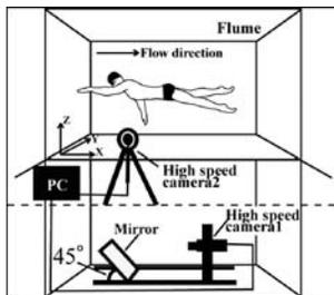
Figure 2. Experimental configuration of the motion analysis.
