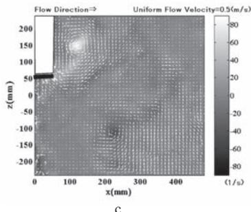
Fig. 4. Sequential variation velocity and vorticity fields in downward motion (viewed from side,  $x$ - $z$  plane). The sampling period is 67 ms or 15 Hz. The mean velocity was subtracted in the velocity vectors.
