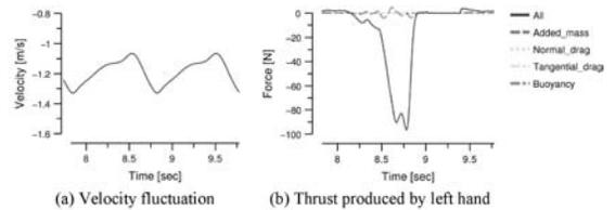
Figure 6. Velocity fluctuation and thrust produced by left hand during one cycle.
