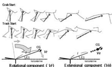
Figure 1. The pendulum model diagram. The starting movement was modeled as a movement including the rotation of segment  $l$  around the front edge of the starting block (rotational component:  $V_r$ ) and expansion-contraction of segment  $l$  (extensional component:  $V_e$ ). The body angle ( $\theta$ ) represents the angle between the segment  $l$  and horizontal line.
