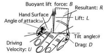
Figure 3. Forces and velocities acting on hand paddle.
