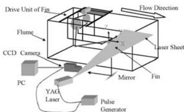
Figure 2. Experimental configuration (horizontal).
