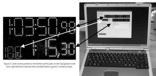
Figure 2. Leds screen on the bottom of the pool on the top (green) total time, right-bottom (red) lap time and left-bottom (green) number of laps.
